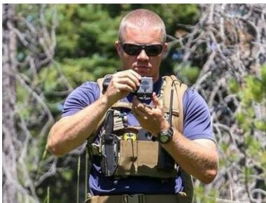
[Cammenga 27CS](#) Lensatic Compass. This is the same compass as the 3N but without the Tritium microlights. For those who want to save \$20, the 27CS is an almost-as-good option. It is equal to its counterpart in accuracy and durability. It only lacks the expensive-to-produce Tritium microlights. But since this model uses phosphorescent glow-in-the-dark paint rather than Tritium, it does not qualify for sales to the U.S. military. Therefore, the NSN validation is not cast into the case.
